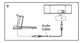
C. Plug one end of the audio cable into the jack beneath the console. Plug the other end of the cable into a 3.5mm Y-adapter (available at electronics stores). Plug the Y-adapter into the PHONES jack on your stereo. Plug your headphones into the other side of the Y-adapter.
